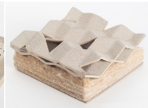
Fabrication: CNC milling and thermoforming
